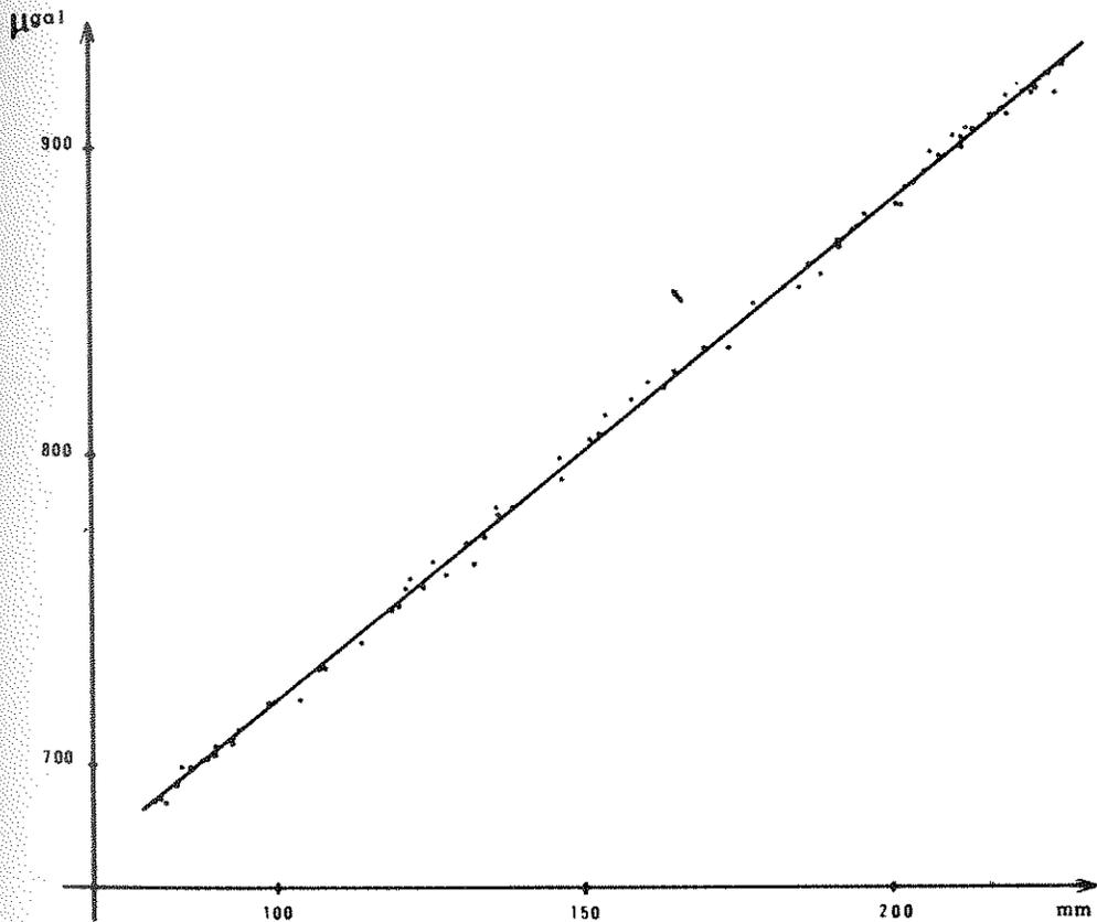
Fig. 1 - Relationship between paper records (in mm) and direct reading values (in  $\mu\text{gal}$ ) of gravity variation measured by the LCR D 40.
