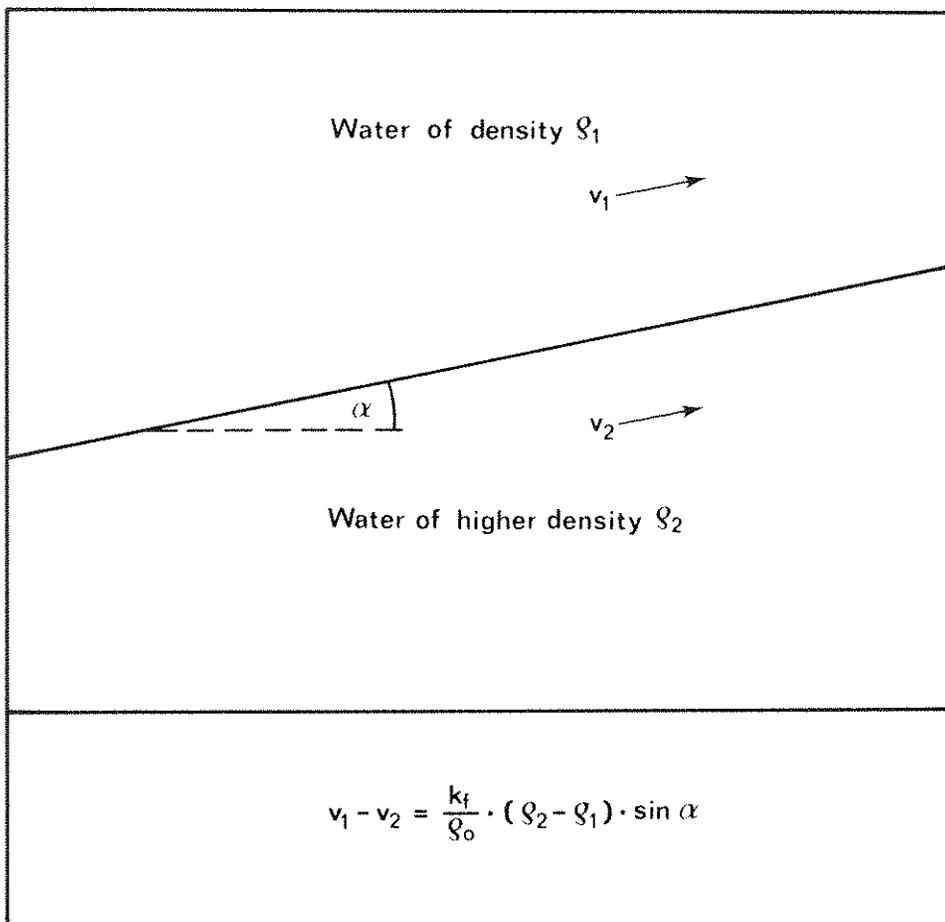
Fig. 8 - Velocity discontinuity at an interface between waters of different density.
