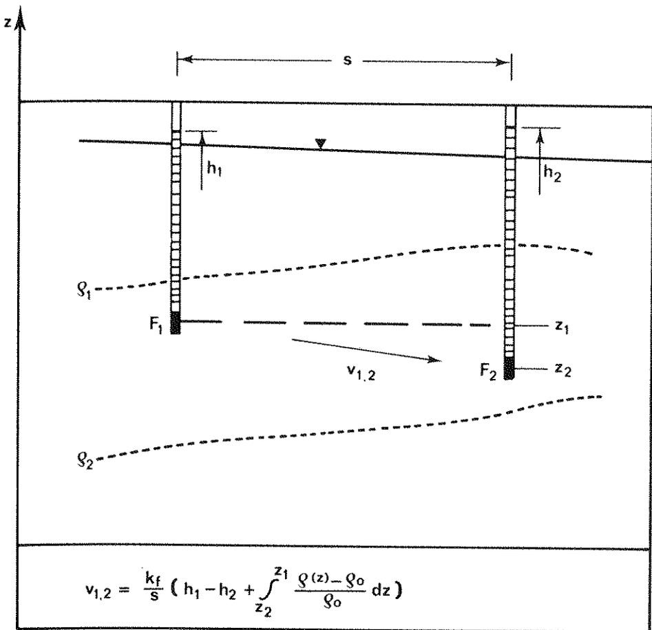
Fig. 5 - Piezometers in groundwater of varying density  $\rho$ . Fresh water with density  $\rho_0$  assumed in the piezometers,  $v_{1,2}$  = Darcy-velocity.
