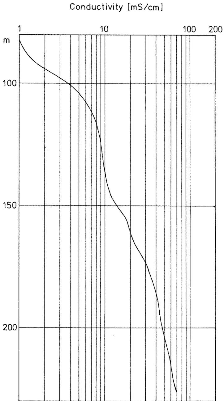
Fig. 4 - Computed log of groundwater conductivity.
