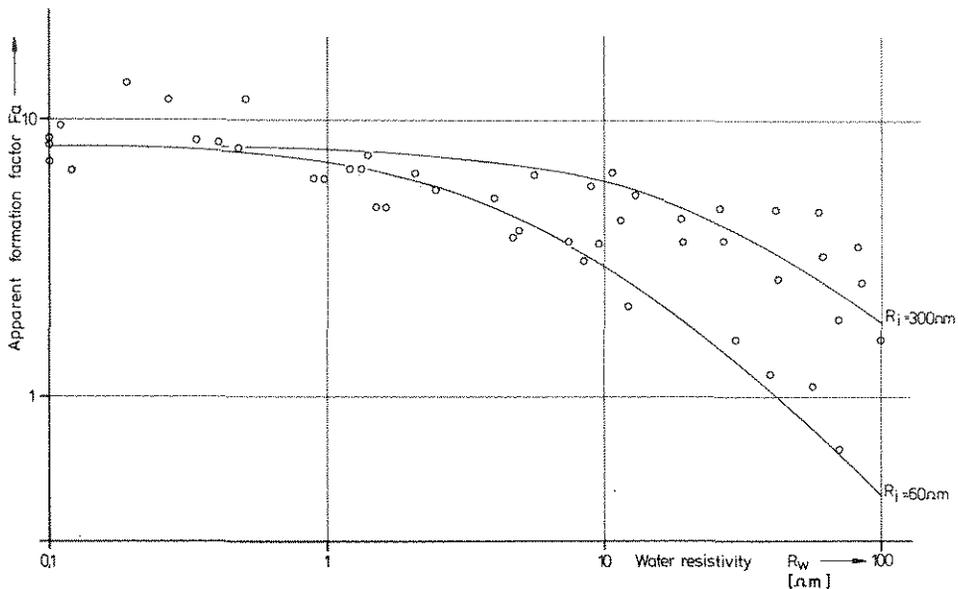
Fig. 2 – Apparent formation factor in relation to water resistivity. The data refer to quaternary sands of glacial origin and varying silt content.
