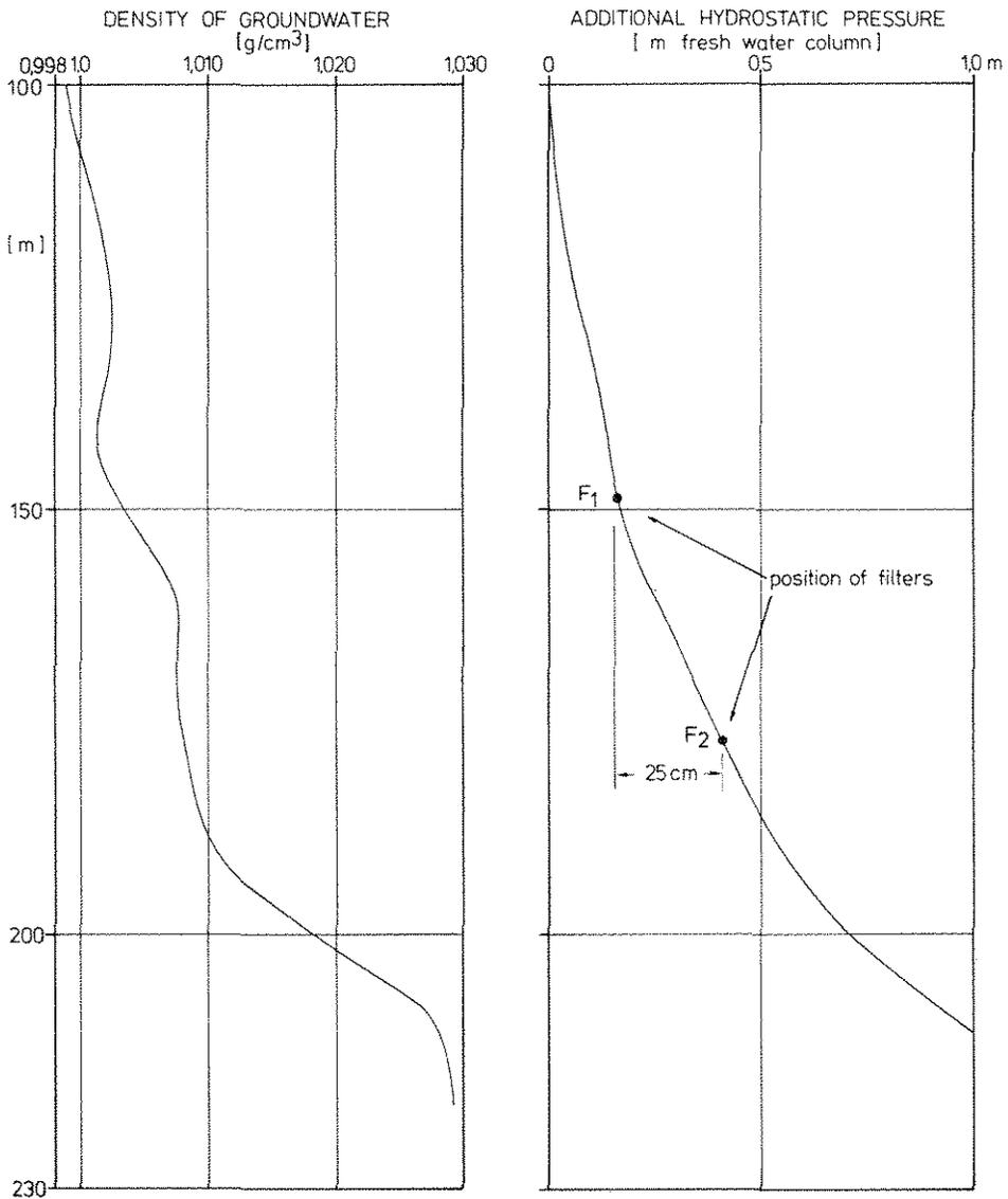
Fig. 6 - Computed logs of water density and excess hydrostatic pressure.  $F_1$  and  $F_2$  are filter positions of two boreholes.
