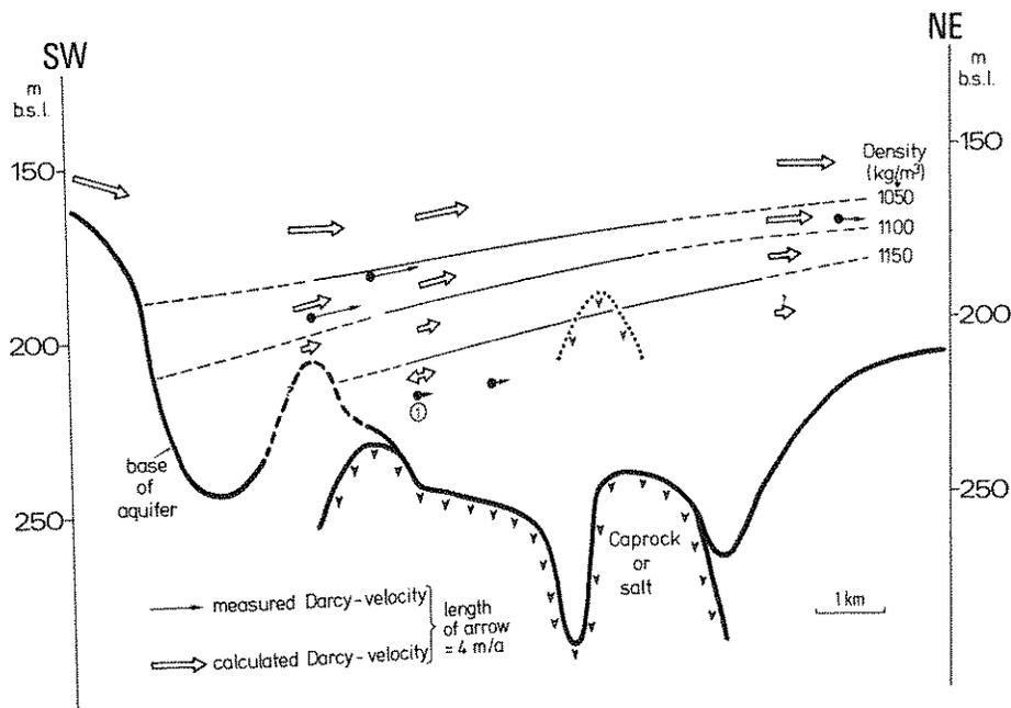
Fig. 7 - Section through aquifer on top of a salt dome, density and velocity of saline groundwater.
