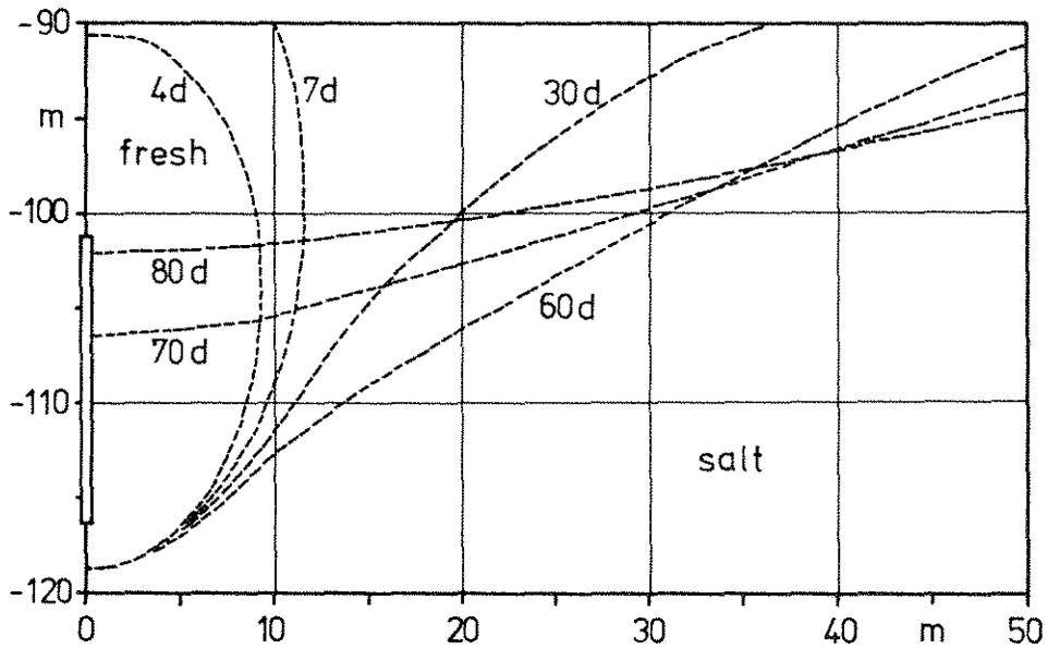
Fig. 6 - Motion of interface if fresh water is injected for 60 days.
