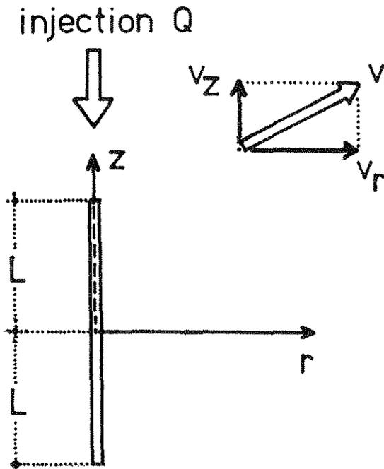
Fig. 5 - Velocity components of flow due to well recharge or abstraction.
