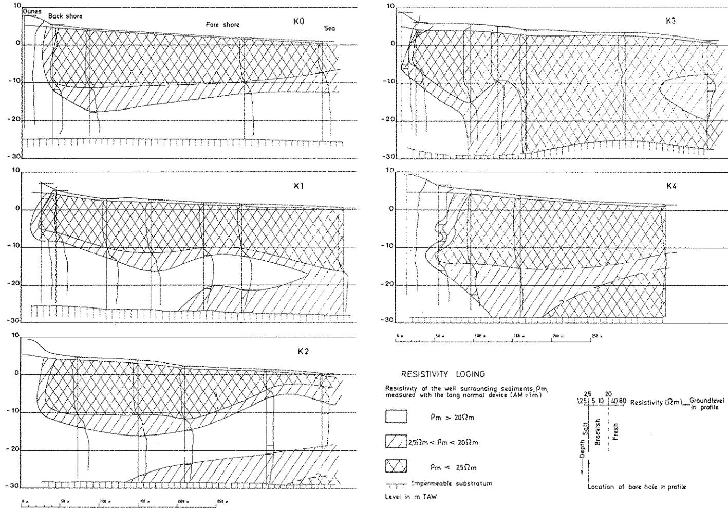
Fig. 2 - Resistivity profiles perpendicular to the shore line of the Westhoek area.
