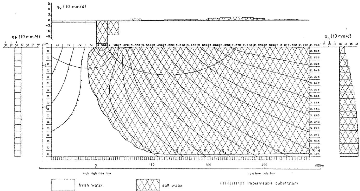
Fig. 4 - Flow of salt and fresh water and the lines of equal fresh-water head with a landward fresh-water flow of 0.09 m<sup>2</sup>/d.
