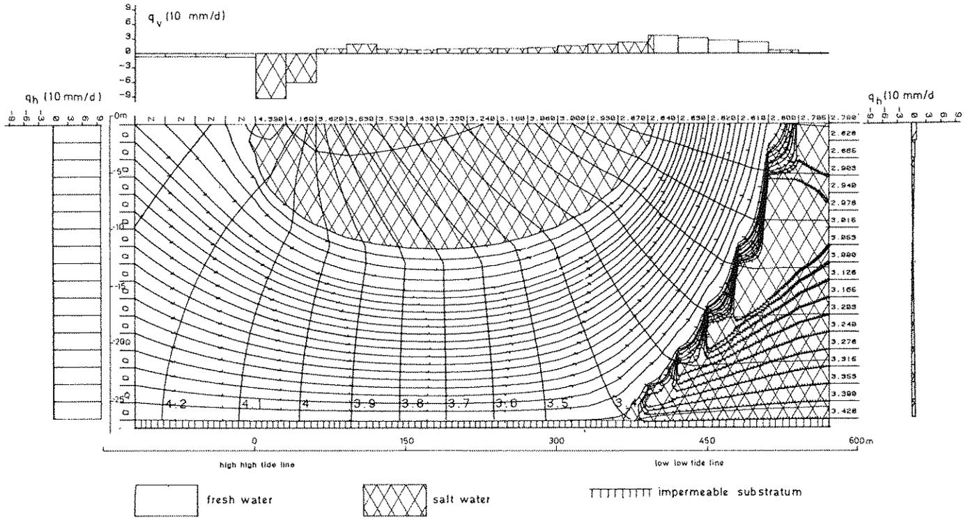
Fig. 3 - Flow of salt and fresh water and the lines of equal fresh-water head with a seaward fresh-water flow of 0.25-m<sup>2</sup>/d.
