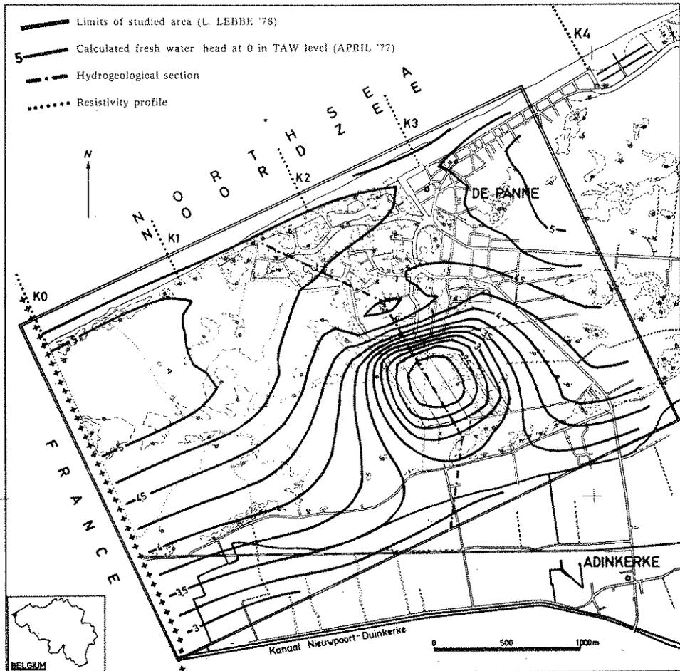
Fig. 1 - Situation of the hydrogeological study in the Westhoek area with calculated lines of equal hydraulic head and of the resistivity logging profiles.
