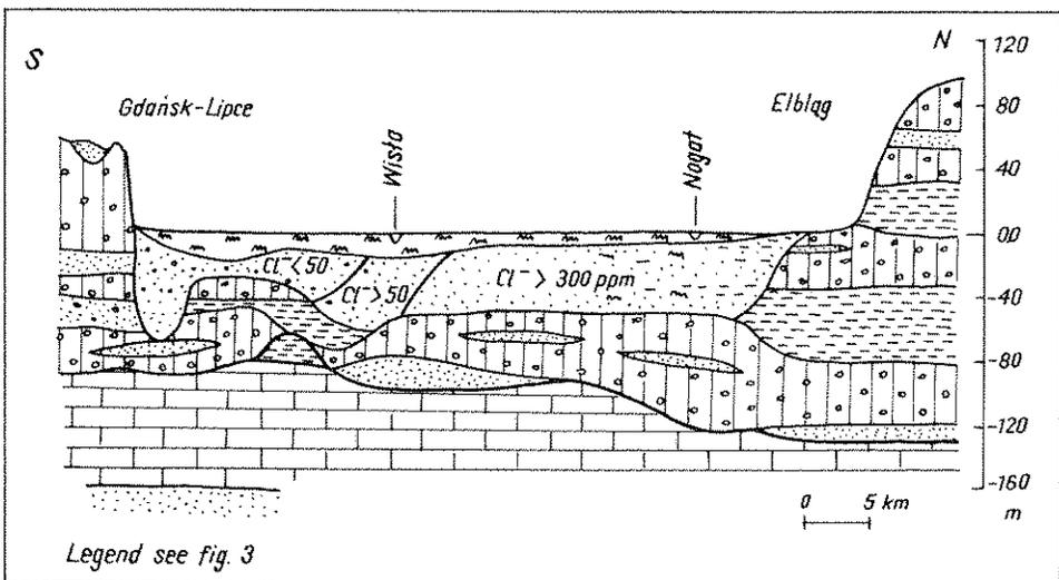
Fig. 6 - Schematic geological cross-section.
