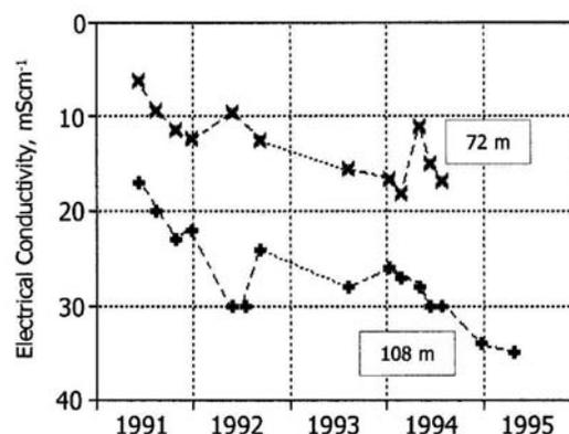
Figure 5: Evolution of electrical conductivity in borehole 224RM at depths below sea level of 72 m (inside the main flow tract) and 108 m (inside the saline water flowing upwards from below). After Domínguez (2000).
