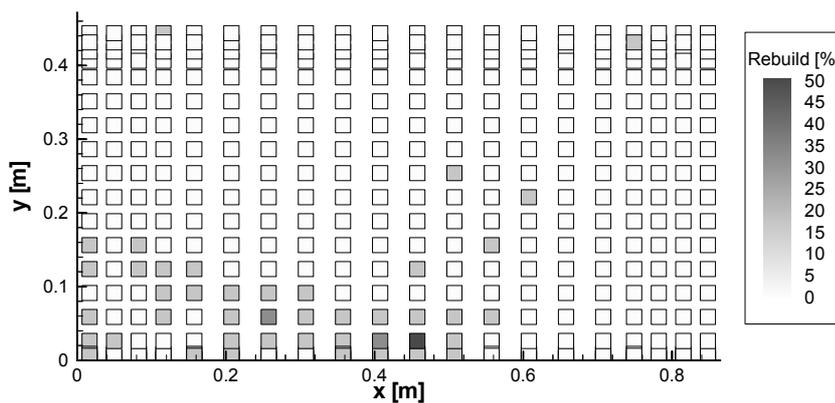
**Figure 3** Distribution of performed matrix recalculations for a single time step, relative to the number of recalculations for the standard approach. Mainly matrices near the head of the saltwater front are recalculated.
