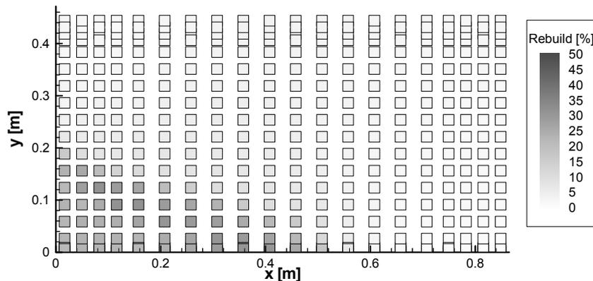
**Figure 4** Distribution of accumulated matrix recalculations for all time steps, relative to the number of recalculations for the standard approach.
