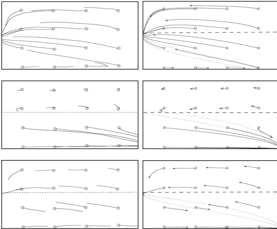
**Figure 2** Experimental (left pictures) and numerical (right pictures) results showing pathlines extracted from tracer movement. The location of the water table is marked by a dashed line. The dotted isoconcentration lines show computed 10% and 90% isosalinities.
