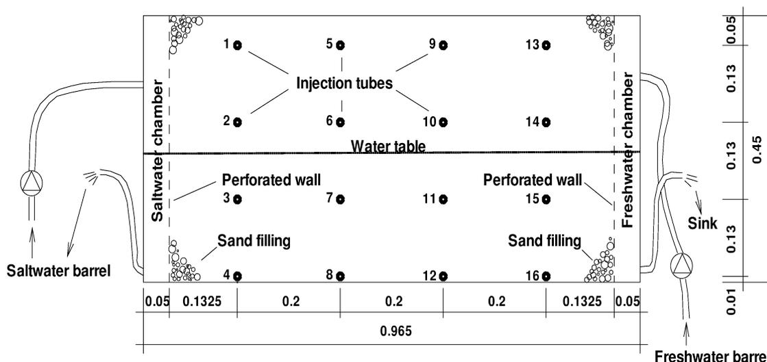
Figure 1 Geometry of the sandbox.
