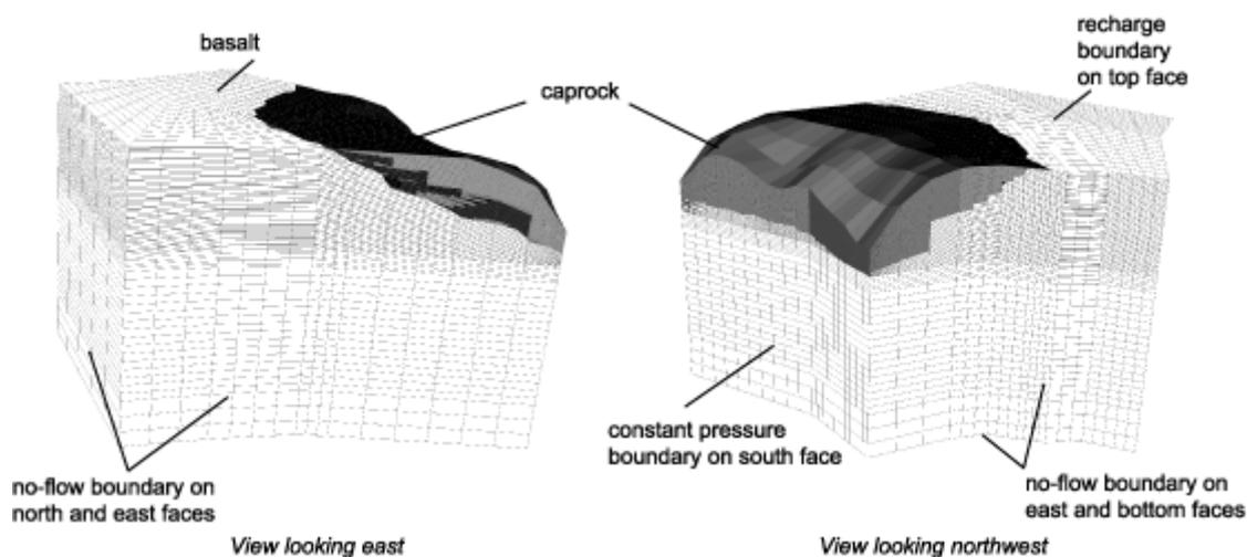
**Figure 4** Three-dimensional views of finite-element mesh used in the ground-water model of the Pearl Harbour area, Oahu, Hawaii. Ocean floor bathymetry is digitized from the USGS 1:100,000 topographic map of Oahu. The elevation of the top of the basalt beneath the caprock is based on contours digitized from Visher and Mink (1964, Figure 6) [onshore] and Gregory (1980, Figure 2) [offshore].
