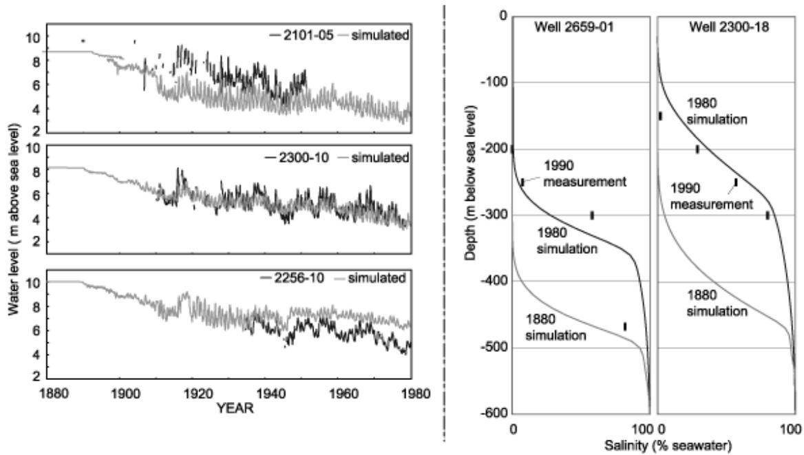
**Figure 5** Simulated water levels and salinity profiles compared with measured water levels (1880-1980) and measured salinity profiles (1990).
