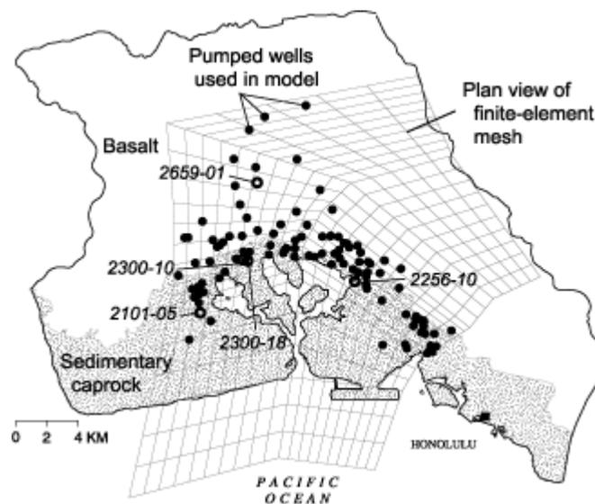
**Figure 3** Extent of sedimentary caprock, pumped (solid circles) and observation wells (open circles), and the finite-element mesh used in the ground-water model of the Pearl Harbour area, Oahu, Hawaii.
