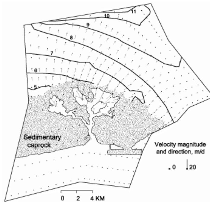
**Figure 7** Velocity vectors (projected to horizontal) at 50-m depth and simulated water-table elevation (solid contour lines in m), 1980.
