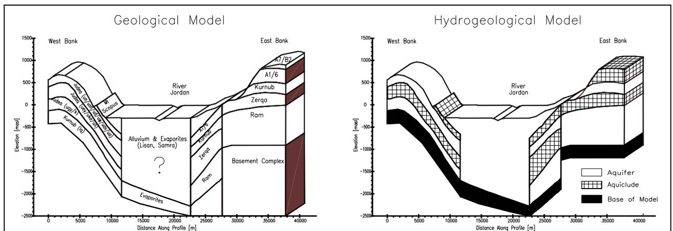
Figure 2 Geological and hydrogeological model of cross section 1 (Modified after Klingbeil et al, 2000)
