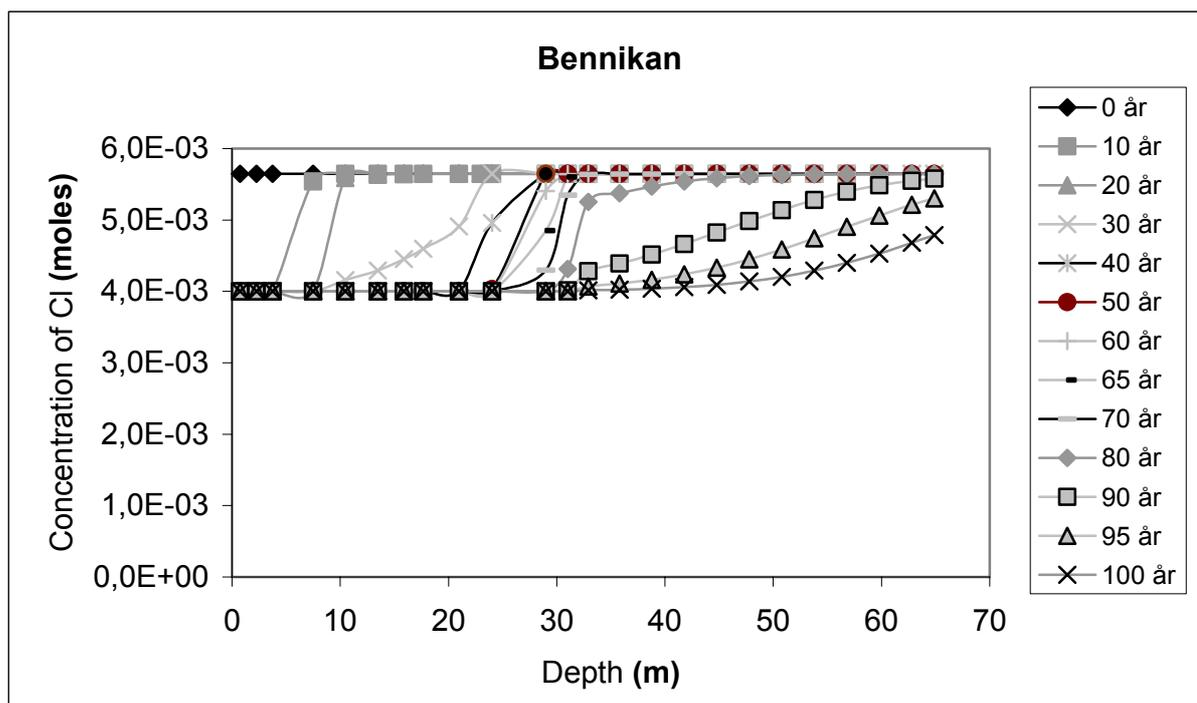
**Figure 6a** The chloride front in Bennikan after modelling a 100-year-outwash with PHREEQC2.0. The front is shown after certain time lengths according to the legend.
