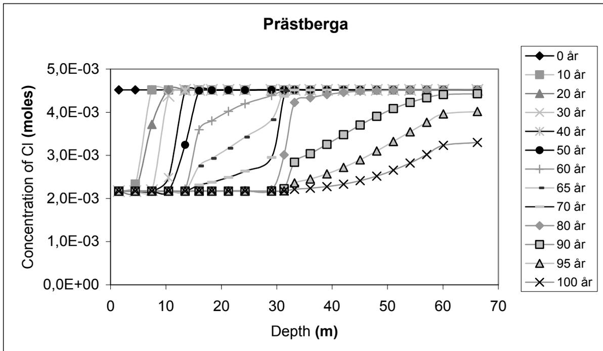
**Figure 6b** The chloride front in Prästberga after modelling a 100-year-outwash with PHREEQC2.0. The front is shown after certain time lengths according to the legend.
