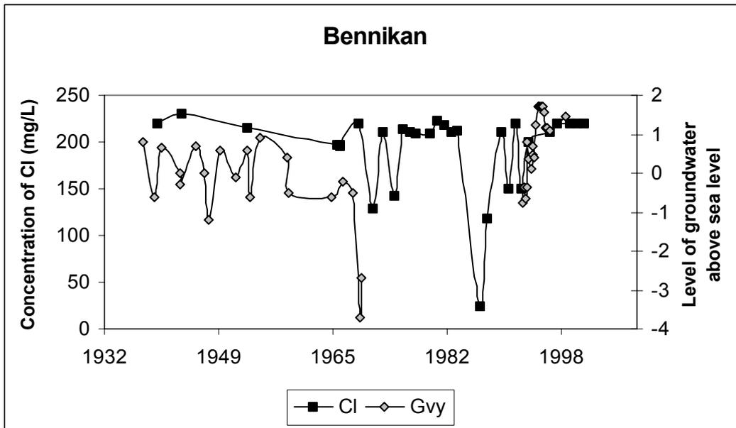
Figure 4 The chloride concentration and groundwater level in the well Bennikan.
