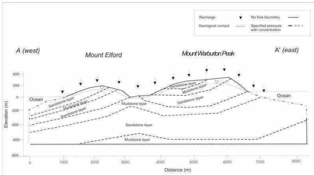
Fig. 6. Cross section across the Saturna Island (A-A') showing hydrostructural domains and relevant boundary conditions.
