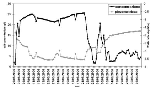
Figure 11: Temporal change of conductivity in the constantly monitored piezometer no. 2
