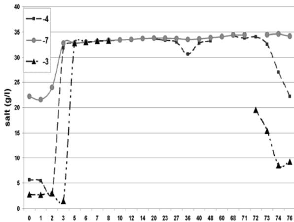
Figure 12: vertical profile of conductivity in piezometer 1
