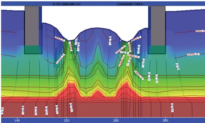
figure. 15 simulations of the situation with barriers inserted into the ground down to a depth of about 6 meters.
