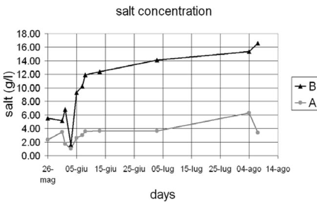
Figure 10 Temporal change of conductivity of the discharge waters of the wellpoint
