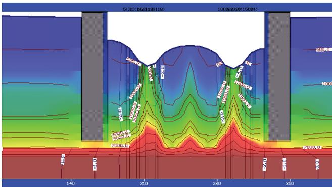
Figure. 16 simulations of the situation with barriers being inserted into the ground down to a depth of about 10 meters
