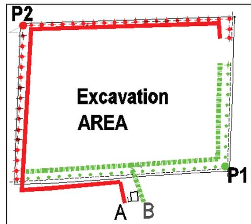
Figure 8: Arrangement of the wellpoints
