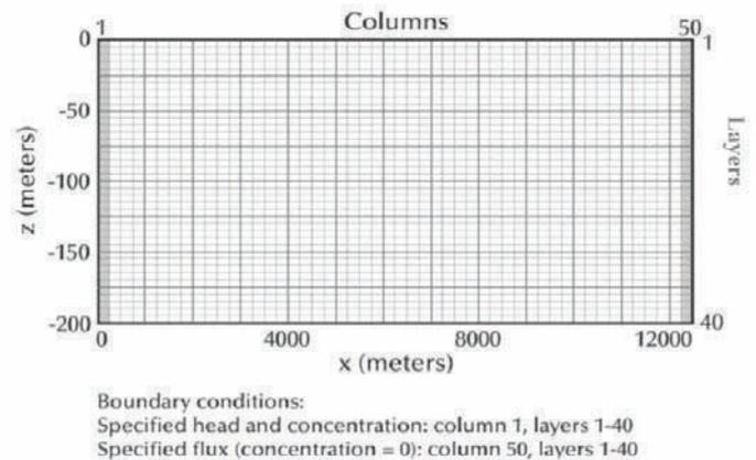
Fig.1. Finite-difference grid used for numerical experiments.
