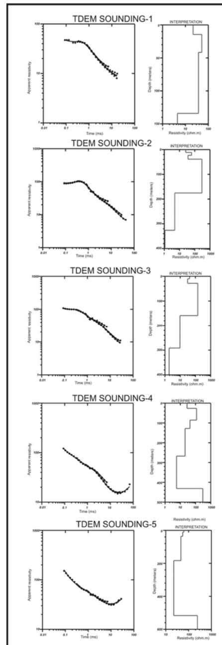
Fig 3. Apparent resistivity curves and interpretation associated
