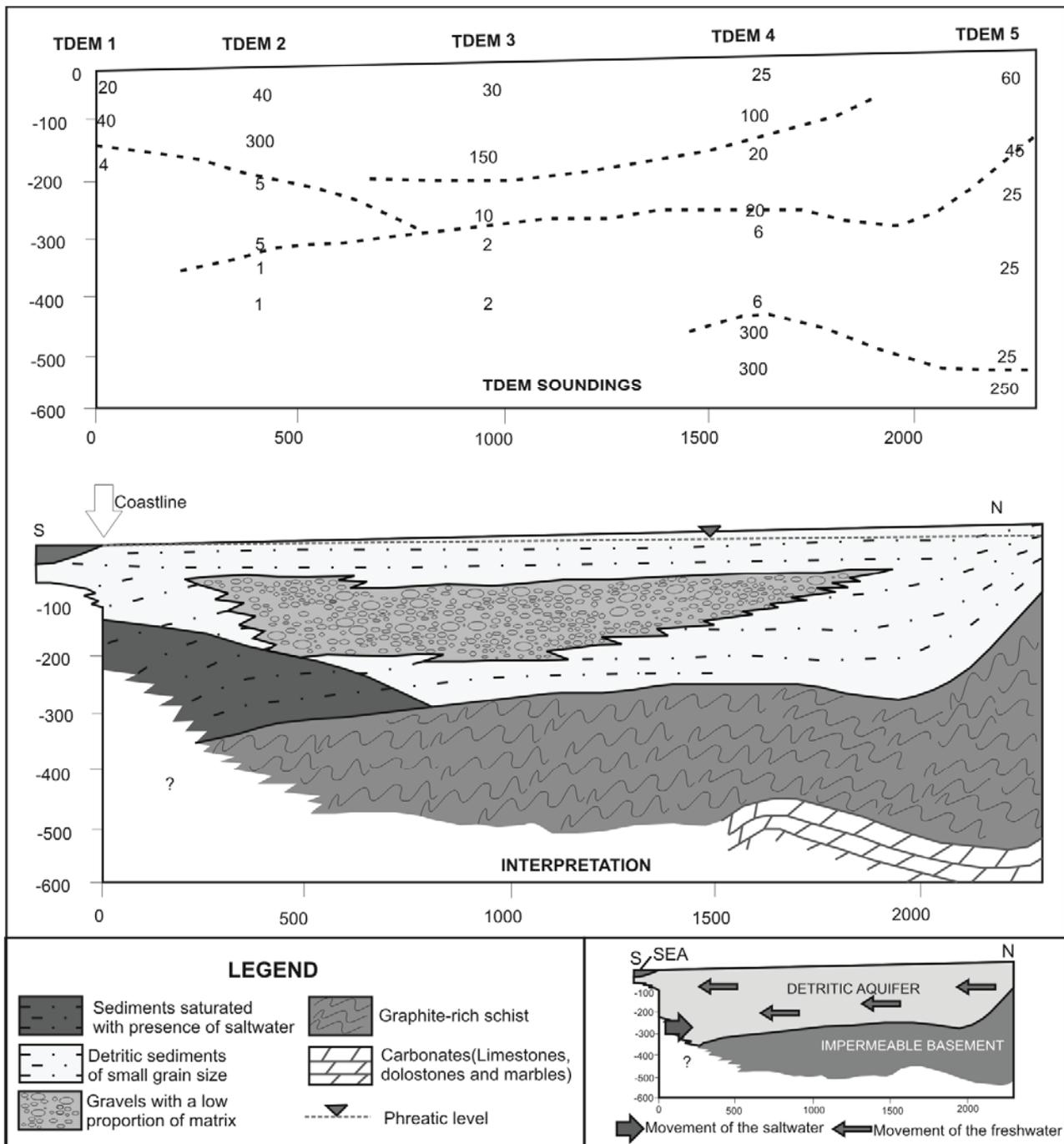
Fig. 4. Section with the electromagnetic data projected and main changes. For the interpretation we have assigned to the units the lithological characteristics of the rocks or sediments that outcrops nearby
