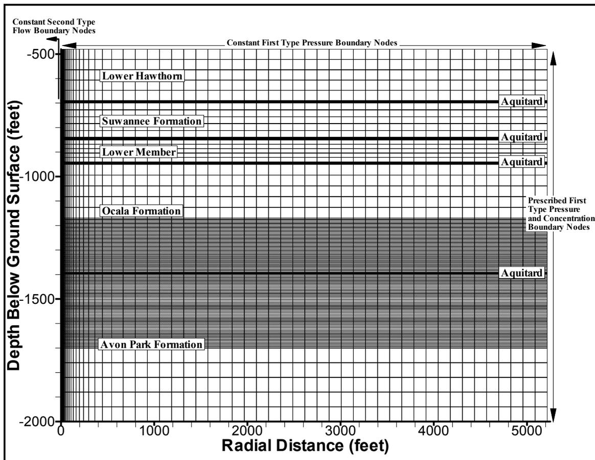
**Figure 1. Model Grid (axisymmetric) and Boundary Conditions**
