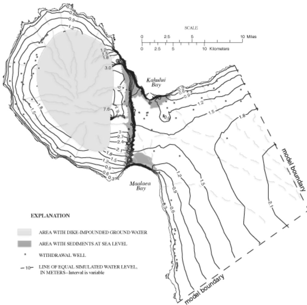
**Figure 2. Simulated water-table contours in 2005, Maui Hawaii, USA.**
