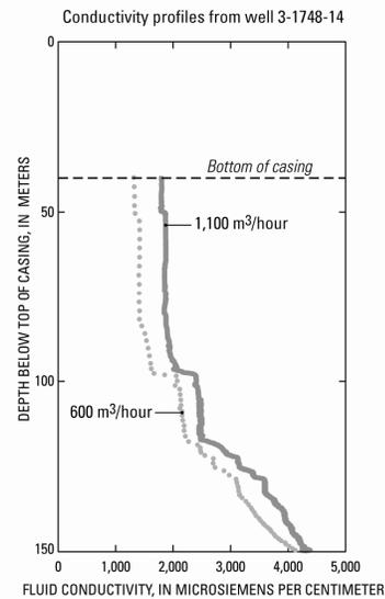
**Figure 3. Fluid-conductivity profiles for nearby withdrawal of 600 m<sup>3</sup>/hour and 1,100 m<sup>3</sup>/hour, southern Oahu, Hawaii.**
