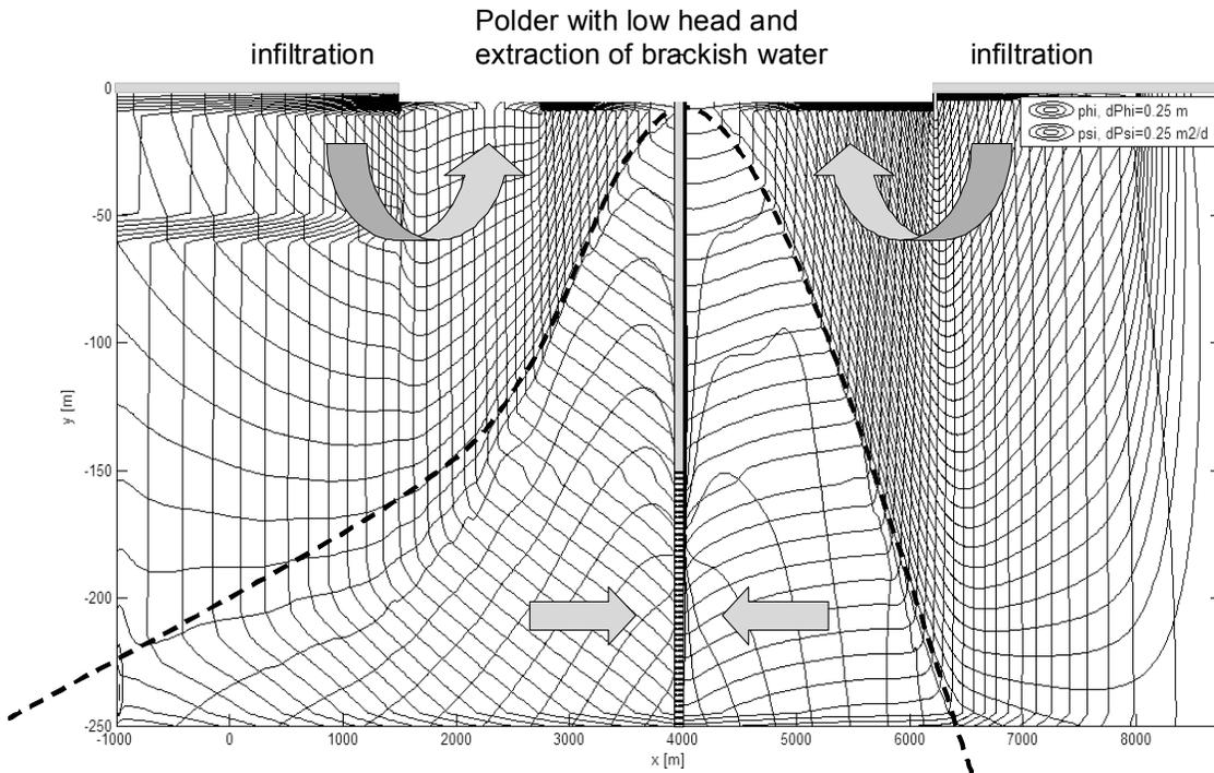
**Figure 2. Cross section now including recovery of brackish water with a line of wells screened between 150 and 200 below ground surface. The equilibrium interface is indicated by the thick dashed lines. Interval between streamlines is  $0.25 \text{ m}^2/\text{d}$ , between fresh water head lines it is  $0.25 \text{ m}$ .**
