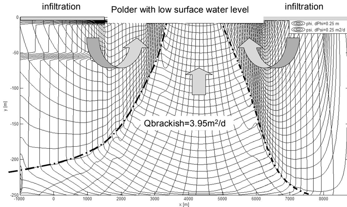
**Figure 1. Cross section with brackish water upconing and seepage in the center. Streamlines at  $0.25 \text{ m}^2/\text{d}$  intervals and fresh water heads at  $0.25 \text{ m}$  intervals are shown. The interface between brackish and fresh water is indicated by the thick line. The brackish water had  $1010 \text{ kg/m}^3$  density.**
