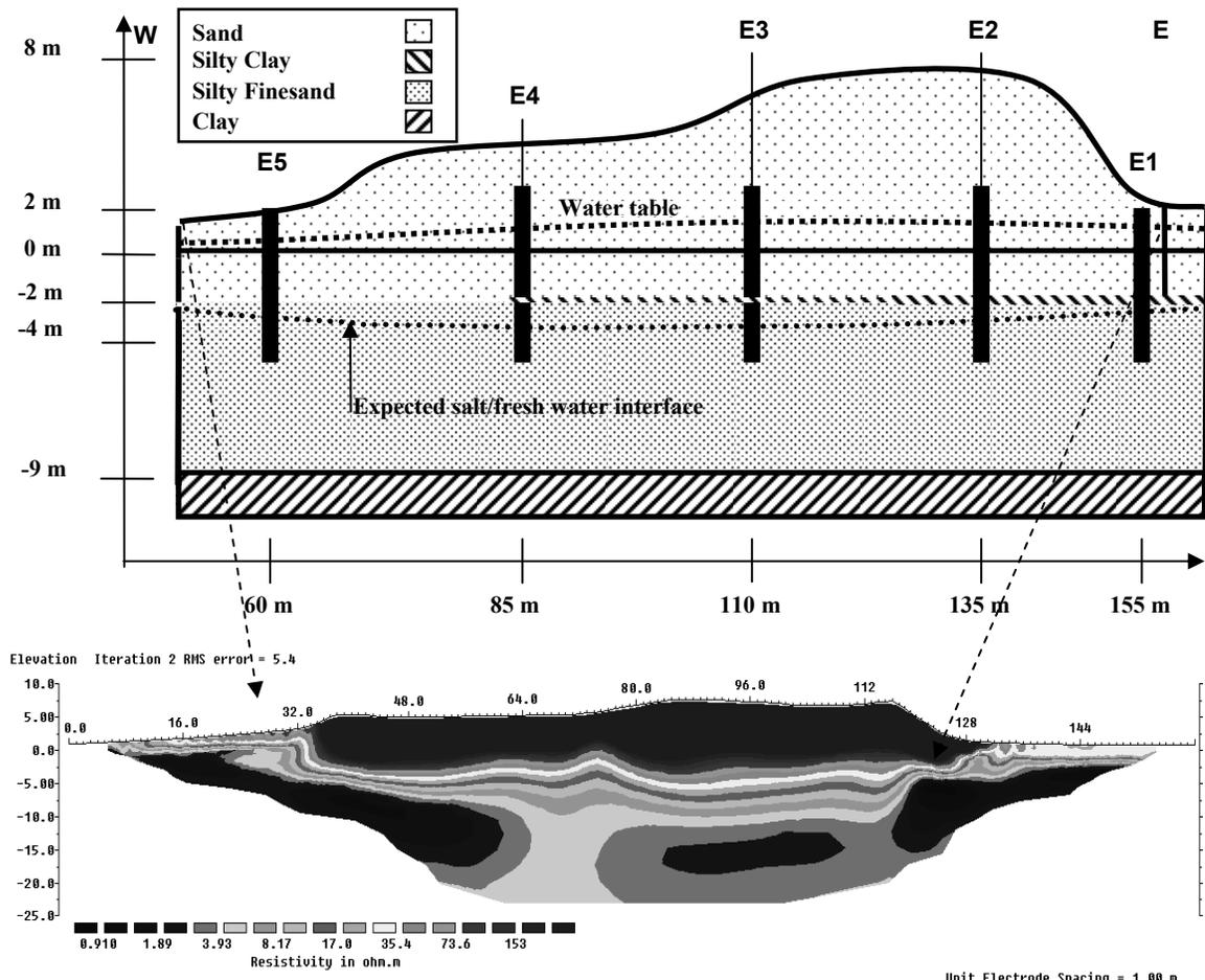
**Figure 1: a) Schematic overview of the profile with MEP-probes E1-E5. X-axis: approximate distance the coastline [M]. Y-axis: Elevation DNN [m]. b) Interpretation of a horizontal MEP profile along the E1-E5. The North Sea is to the west, the lagoon area is to the east.**
