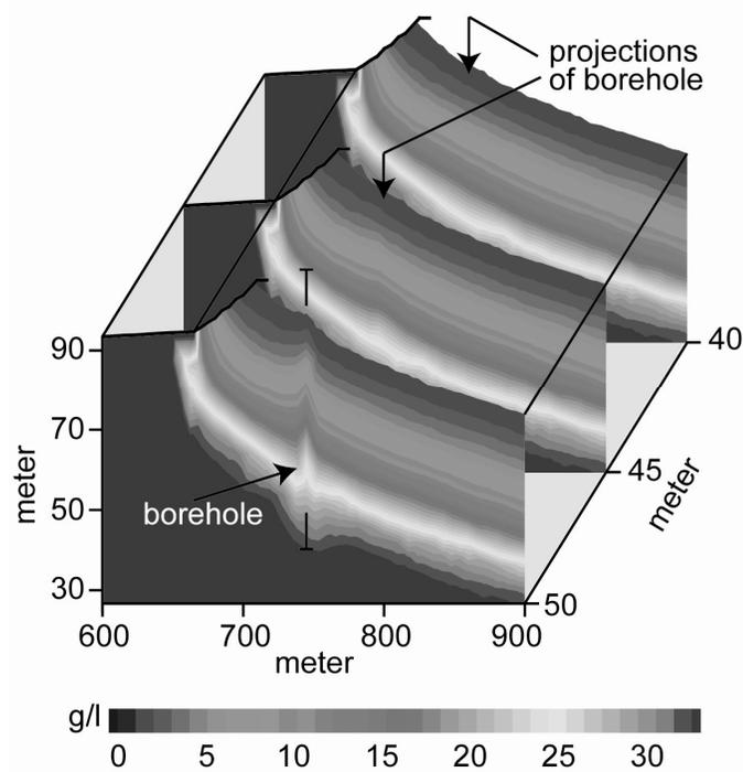
**Figure 1.** Simulation results showing salinity distribution around the borehole for the anisotropic case. The borehole affects the natural flow and elevates the freshwater-saltwater mixing zone. Away from the borehole the natural flow is undisturbed.
