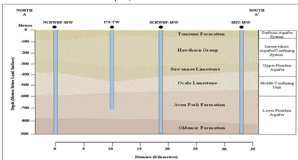
Figure 2. Hydrologic Cross-Section from A to A' through Naples, Florida (line of cross-section shown in Figure 1.)
