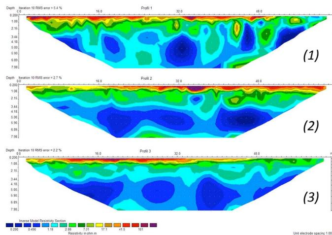
Figure 2. Surface electrical profiles obtained in a triangle oriented along a NE-SW strike from MAG1 (Profile 1), a NE-SW strike from MAG4 to MAG1 (Profile 3), and NS for that closing the triangle (Profile 2). Vertical penetration does not exceed 8 m depth.
