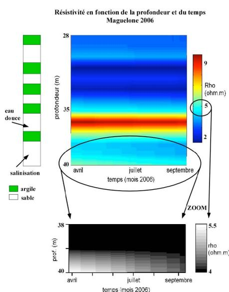
**Figure 4. Automated measurement of electrical resistivity as a function of depth (from 28 to 40 m) in MAG-4 and time (from April to September 2006), with simplified lithology to the left indicating the presence of clay layers (bright green), and zoom at bottom on resistivity changes as a function of time in the bottom two meters, showing a gradual salinisation.**
