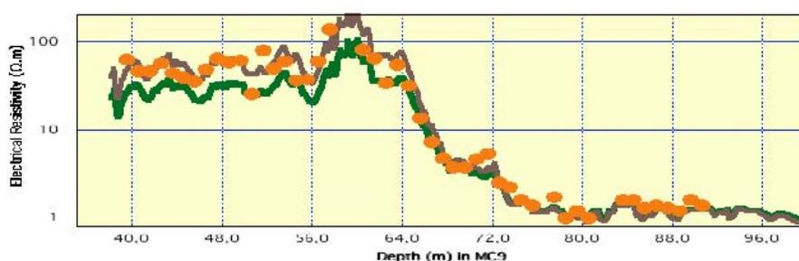
**Figure 5. Measurement of electrical resistivity as a function of depth (from 40 to 100 m) in Hole MC9 (Campos, Mallorca, Spain), showing that recorded with the downhole stringer (yellow dots) in comparison to that obtained with an induction resistivity tool (green and brown profiles for deep and medium sounding into the formation, respectively).**
