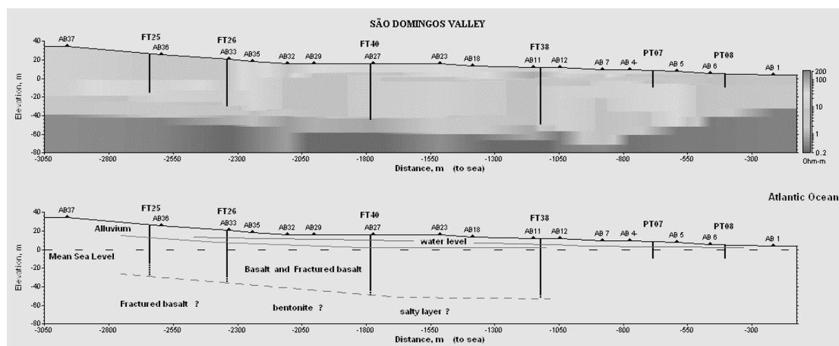
**Figure 4. Geoelectric pseudo-section at S. Domingos creek valley (June 2005), with TDEM soundings and boreholes location. Lithology is drawn from boreholes information.**
