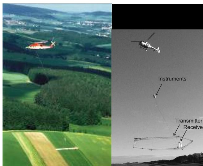
**Figure 2. Helicopter-borne geophysical systems: Left: BGR system recording simultaneously frequency-domain electromagnetic, magnetic and radiometric data, Right: SkyTEM system recording time-domain electromagnetic data.**
