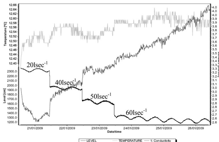
Figure 1. Step Pumping Test at Cork South Docklands from 20/01/2009 – 28/01/2009
