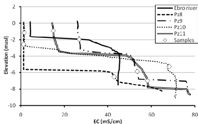
Figure 3. EC Vertical profiles for one line of piezometers (Dec-2009).
