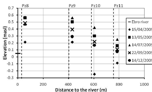
Figure 2. Evolution of the piezometric level versus distance to the Ebro River.
