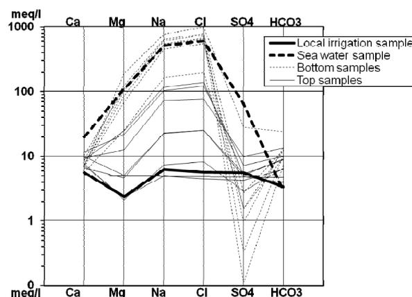
Figure 4. SCHOELLER-BERKALOFF chart where samples from the irrigation channel, sea water and the top and bottom of the piezometers are differentiated.
