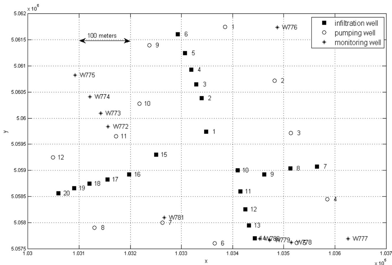
Figure 1. Layout of the ASR system
