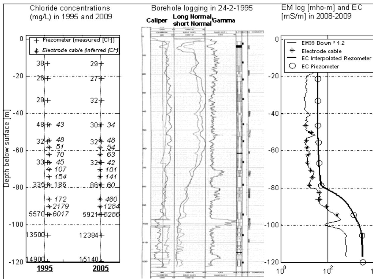
Figure 2: Comparison of [Cl-], electrode cable (left), SN/LN and caliper/gamma logs (center), and EM-log / EC / electrode cable (right) for well 24H718
