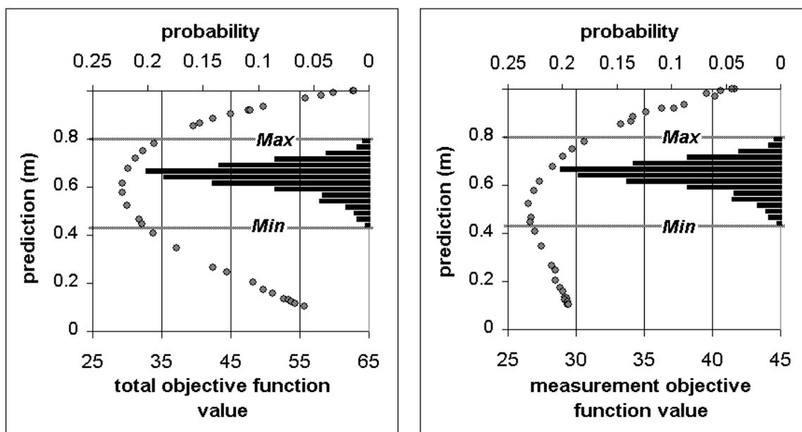
Figure 2 Prediction versus the total objective function value (left) and prediction versus the measurement objective function associated with the available concentration and head observations (right). Results of the uncertainty analysis with DREAM are indicated by the histogram and the lines Min and Max.
