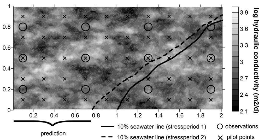
**Figure 1 Stochastic hydraulic conductivity field, locations of pilot points and observation data. Position of the 10 % seawater line indicated before and after reducing the freshwater flux in stress period 2.**
