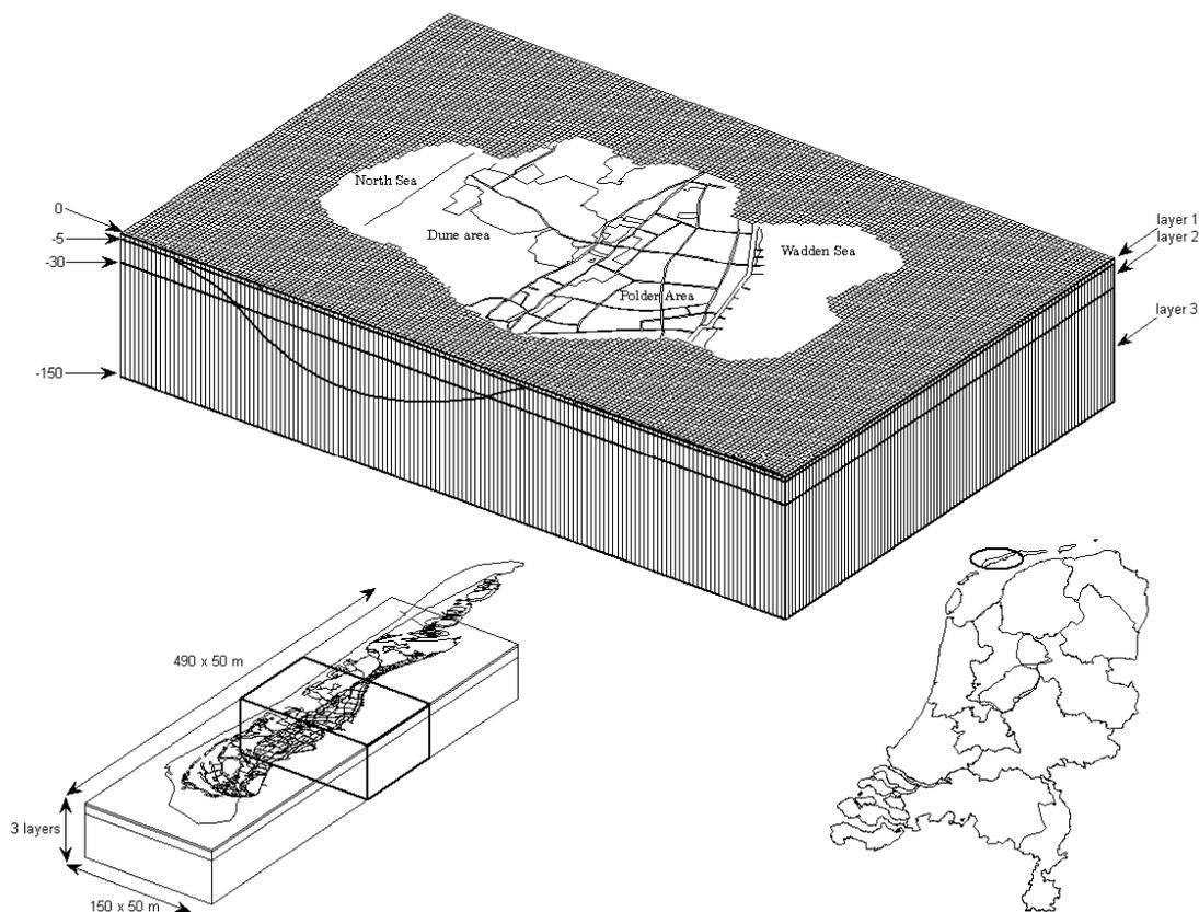
Figure 1. Model setup: 3 layers, 150 rows, 490 columns. 50\*50 meter gridsize.
