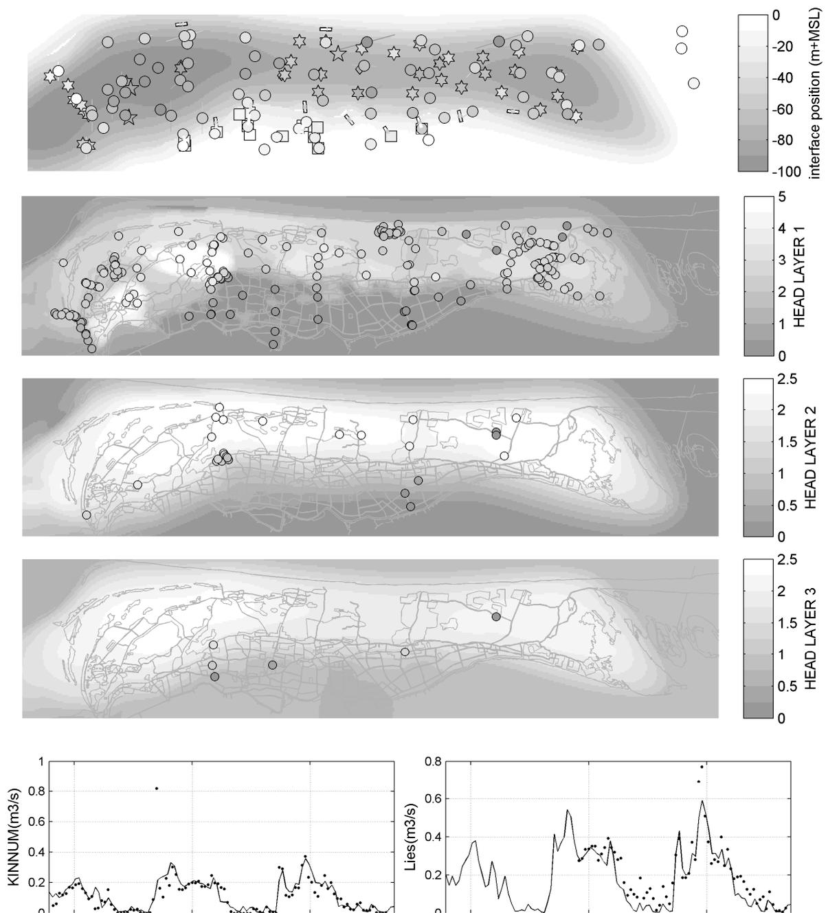
**Figure 2. Calibration results from top to bottom: maps of interface depth and head in layer 1 to 3. Symbols are point measurements, background is the model result. The bottom two graphs are the discharge from two polders as a function of time. Measurement points versus model result (continuous line).**
