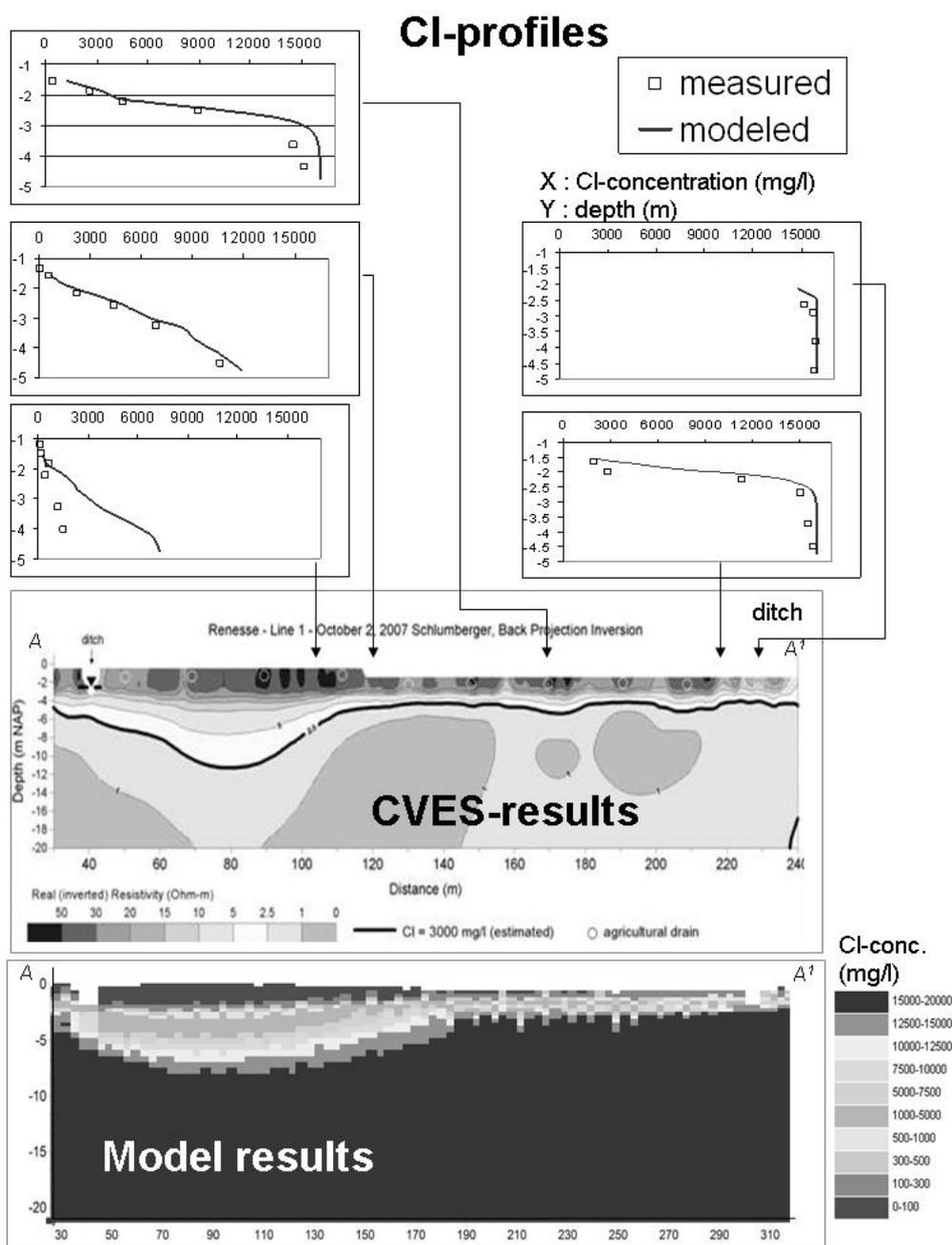
Figure 2. Top: Modeled and observed chloride profiles. Center: CVES-results in cross-section A-A<sup>1</sup> (from De Iouw *et al.*, 2008). Bottom: Modeled chloride concentration in cross-section A-A<sup>1</sup>.
