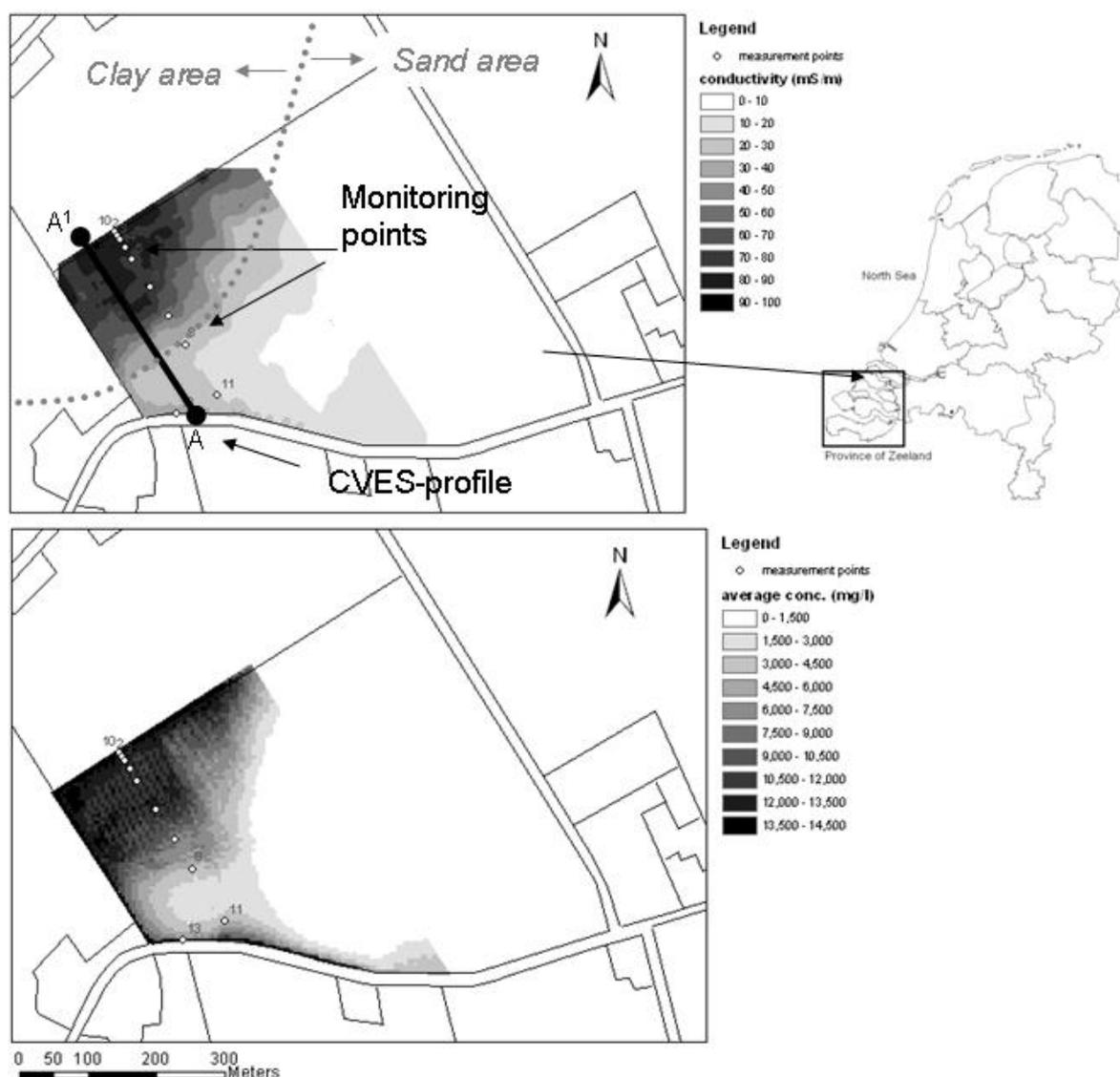
**Figure 1.** EM31-conductivity values for the upper 6m (top). Modeled average chloride concentration of the upper 6m (bottom). CVES-line and monitoring point are indicated in the top-picture.
