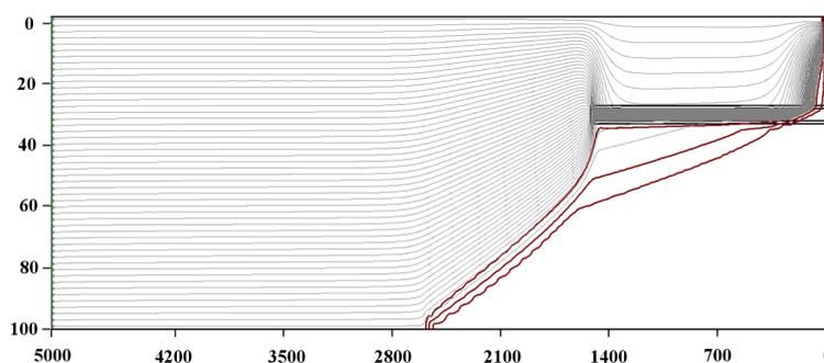
**Figure 2. Groundwater streamline with the presence of high permeable layer.**
